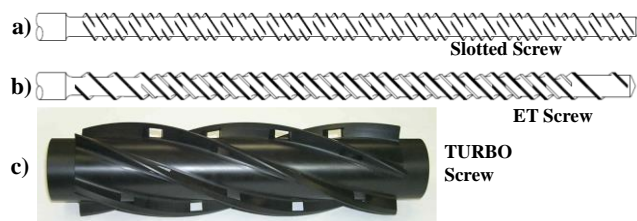
Figure 4. Schematics for commercially available screws for the secondary extruder: a) slotted flight design, b) four channel ET screw design (courtesy of Jeff A. Myers of Robert Barr, Inc.), and c) a segment of a TURBO screw (courtesy of James D. Fogarty of Plastic Engineering Associates Licensing, Inc.)
